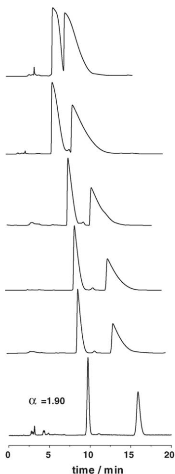
Fig. 10. Loading study of a 250 mm \times 4.6 mm column packed with CSP1. Amount injected in mg, from bottom to top: 0.001, 1, 2, 4, 10, 20 of rac - 6 dissolved in the mobile phase at a concentration of 100 mg/mL (bottom trace: 1.0 mg/mL). Eluent, dichloromethane/methanol 97/3; flow rate, 1.0 mL/min; T = 25^\circ\text{C} ; detections, UV at 350 nm.
